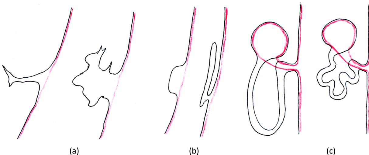
Figure 1: Pairs of scenarios illustrating differences in measured displacement depending on the metric used. Original polylines shown in black, simplified polylines shown in red. (a) approximately equal linear displacement but very different areal displacement, (b) approximately equal Hausdorff distance but very different Fréchet distance, (c) approximately equal shift in areas covered by adjacent polygon features but very different positional displacement of line features.
