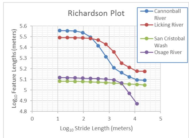
Figure 1. Richardson plot of four linear stream features extracted from 1:24,000-scale National Hydrography Dataset flowline features. Features include the Cannonball River, Licking River, San Cristobal Wash, and the Osage River.
