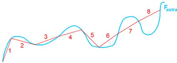
Figure 2. Richardson plot measurements. Set of eight equal-length strides (red) used to estimate “walk” length of stream feature (blue). Left over length of stream beyond the eight strides represented as  $F_{extra}$ .
